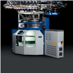
Traditional Orizio modular frame, renovated in its functionality, robustness and aesthetics with the new, integrated 'Oritec' control panel which visibly allows the fruition of new technologies and complete control of the needles selection with the following functions:
