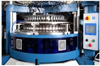
Traditional Orizio modular frame, renovated in its functionality, robustness and aesthetics with the new Orizio ''Oritec'' control panel which allows the fruition of new technologies and completes the machine's control, the needles selection and the following functions:
