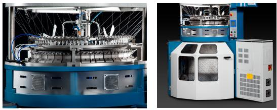
Traditional Orizio modular frame renovated in its functionality, robustness and aesthetics, with the new "Oritec" control panel which allows the fruition of new technologies and completes the machine's control with the following functions:
